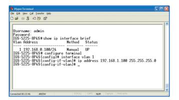
Figure 6-2: Configuring IP Address Screen
