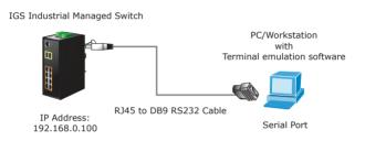
A terminal program is required to make the software connected to the IGS-5225 series Industrial Managed Switch.
