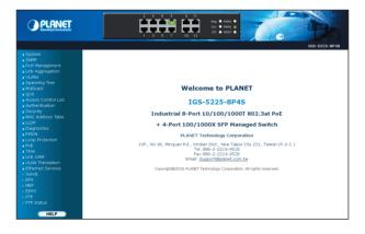
Figure 7-3: Web Main Screen of Industrial Managed Switch
